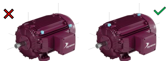
Mounting on cooling fins and covers is not recommended. Note: For motors, it is recommended to mount a sensor on the drive end and another one on the non-drive end for complete monitoring.
