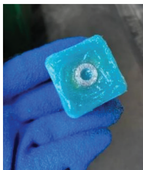
Figure: Glue mount DynaLogger installation DynaPredict Manual - Quick Start Guide - Version 6 – July 2024 Public Document
